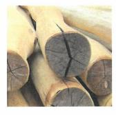
Minor cracks does not affect the strength of the wood and will not require any action. In the event that they conflict with the allowed tolerances described in current safety standards or any other local regulations a repair is necessary according to the maintenance instruction.
