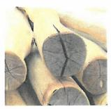
Minor cracks does not affect the strength of the wood and will not require any action. In the event that they conflict with the allowed tolerances described in current safety standards or any other local regulations a repair is necessary according to the maintenance instruction.
