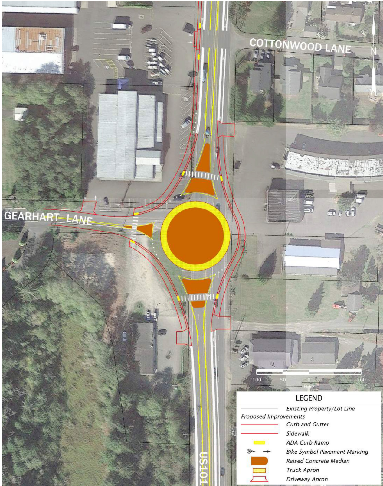
Figure 6-6. Conceptual Roundabout Design at Gearhart Lane (Project R-2b)
